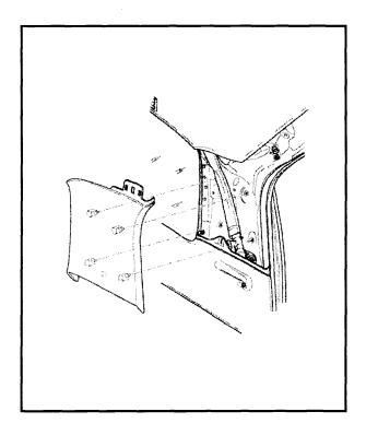
Pull D-pillar trim out of mountings in body and door seal molding
