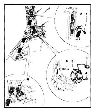
Remove bolt -1- and pull belt relay -2- off belt height adjuster
