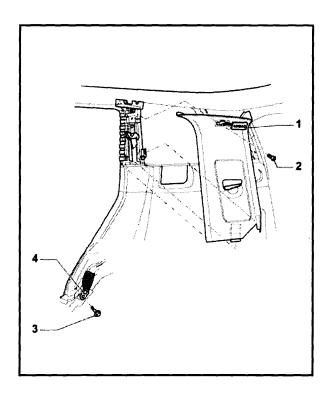
Pull seat belt through opening and reinstall trim into mountings in body and door seal molding
