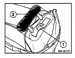
22. Fold the first ply (1) of the heating fleece back over the repair area and seal the repair area with the large fleece adhesive strip (170 mm x 55 mm) (2) provided in the repair kit.
