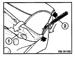
4. Fold down the cotton fabric (1) to gain access to the heating fleece.
