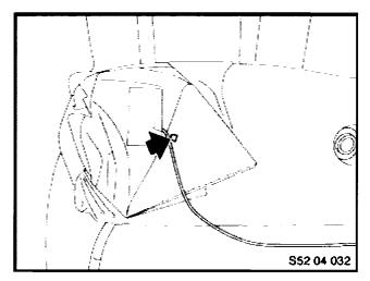
23. Cut a small hole into the padding near the new wire (as indicated by the arrow) and then pull the wire through loosely.
