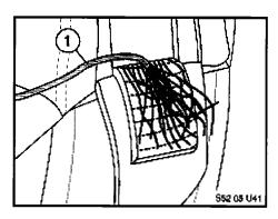
15. Strip the wire (1) from the repair kit (copper-colored end) and fan out the strands. Join the copper strands to the 11 metal heating strands and twist them together.
