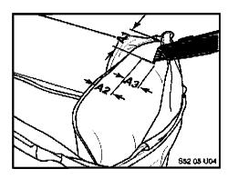
7. Cut open the heating pad along the marking made for dimension A3 to expose all 11 metal strands (1). This cut can be made using a razor or a seam ripper. Note: The heating fleece consists of 3 plies. Be careful when cutting along dimension A3 to only cut into the first ply. The metal strands are bonded to the second ply of the heating fleece.
