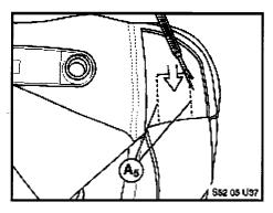
11. Cut parallel incisions (at a distance of 10 mm) to the left and right of the metal strands. Only cut into the first ply of the heating pad.
