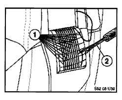
13. Carefully pull up on each metal strand (1), using the blunt side of the seam ripper (2), to release them from the fabric threads. Start pulling up on the metal strands near the cut made for dimension A4. Continue until at least 30 mm of each of the metal strands has been released from the fabric threads.
