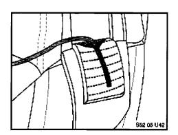
dimension A4. Continue until at least 30 mm of each of the metal strands has been released from the fabric threads.
