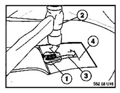
20. Using a hot glue gun, apply glue to the center of the small fleece adhesive strip (1) and affix crimped strands to the glue.
