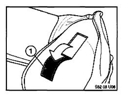
9. Peel back the first ply (1) of the heating fleece 50 mm to expose the metal strands.
