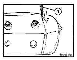
3. Using a seam ripper (1) cut the cloth material open along the marking (dimension A2).
