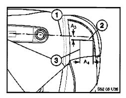
8. Below the guide line (1) made in step 7, draw a second guide line (2) approximately 10 mm below. A3: approximately 10 mm.
