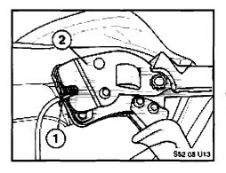
16. Crimp (1) using special tool (2) number 52 0 100. Cut off the protruding strands approximately 5 mm from the end of the sleeve.
