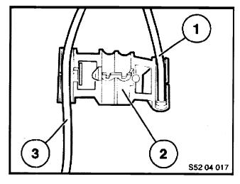
12. Connect blue wire (1) to backrest heating wiring harness (3) using a snap connector (2).
