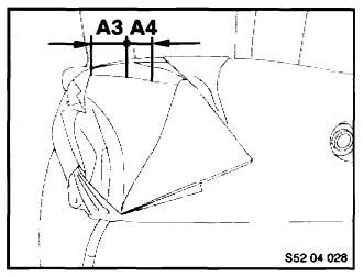
9. Cut open the backrest heating pad along the length of the marking (dimension A4) to expose all 11 metal strands, widen the cut if necessary. Note: Cut into the backrest heating carefully to avoid damage to the cover surface material.
