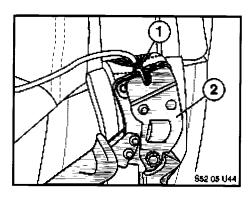
18. Crimp (1) using special tool (2) number 52 0 100. Cut off the protruding strands end of the sleeve.
