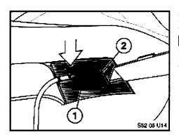
mm x 40 mm), from the repair kit, over the padding where the cuts were made.
