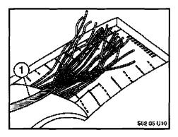
13. Strip the wire (1) from the repair kit (coppercolored end) and fan out the strands. Join the copper strands to the 11 metal heating strands and twist them together.
