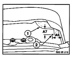
2. Mark (2) the rear side of the foam pad at a distance equal to dimension A7 from the edge of the lower molding contour (1) on the back of the foam pad and mark (2) at a distance equal to dimension A6 from the door side edge.
