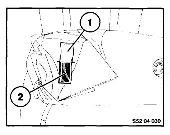
11. Peel back the first ply of the heating pad (1) to expose the metal strands (2).
