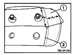
2. Fold the top portion of the seat cover (1) forwards, away from the foam backrest pad (2). Mark the following dimensions on the cloth material of the seat cover (1).
