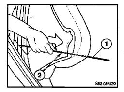
3. Push welding rod (1.5 - 2.5 mm2) (1) up through the two markings from the rear side of the foam pad (2).
