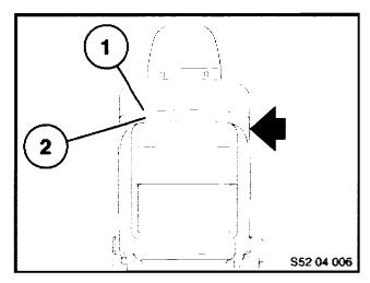
To remove the backrest panel, reach between the backrest panel and the cover in area (1) until you can feel clip (2). Pull the backrest panel to the rear slightly. With your other hand, strike the side of the backrest panel (as indicated by the arrow) from the inboard side of the seat. The clip on the door side is then released from the catch.
