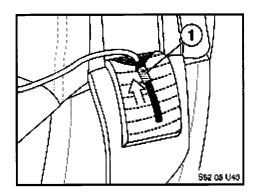
16. Push the crimp from the kit over the twisted strands with the larger diameter first.
