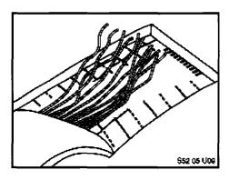
12. Once the 11 metal strands are released from the second ply of material, fan out the strands to make them ready to splice with the wire from the repair kit.
