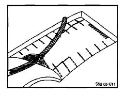
14. Twist the wires together tightly to form one slender splice of both sets of wires.
