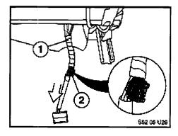
13. Wrap the blue wire and the wiring harness (1) with electrical tape up to the snap connector (2).
