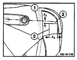
9. Mark dimension A4 from the door-side seam to guide line (3).
