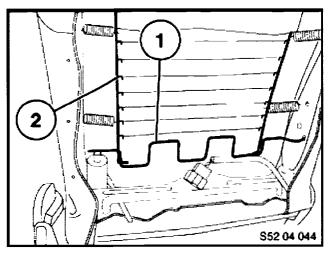
4. Draw the contour of the flexmat (2) and compression spring (1) on the door side with a suitable marker so proper fitment can be checked during installation.
