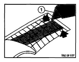
10. Use a razor (1) or a seam ripper to cut across the 11 strands by following the same cut made for dimension A3.
