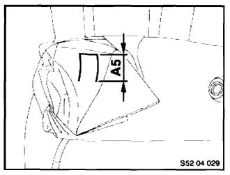
10. From the corners of the cut made above, cut parallel incisions to the left and right of the metal strands.
