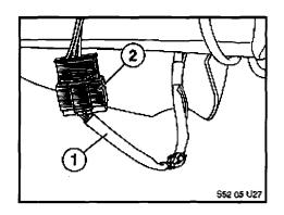
14. Connect the seat heater wiring harness (1) to the seat harness connector (2).
