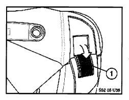
12. Peel back the first ply of the heating pad to expose the metal strands (1).
