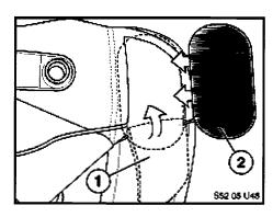
22. Turn the fleece padding (1) up and affix using the large fleece adhesive strip (2) from the kit over the top of it. Route the blue wire loosely on the door side of the seat.
