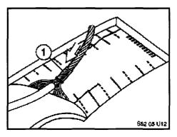
15. Push the end sleeve (1), from the repair kit, over the twisted splice.
