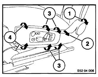
Unclip the trim at the sides (1) to the rear, pull it upwards, then pull the belt opening to the side (2).
