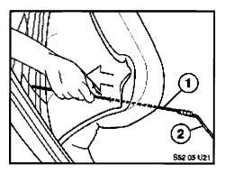
4. Bend upper section of welding rod (1) into a small loop and fasten the wire (2) to it. Pull the wire and welding rod through the foam pad blue end first. Note: Route the blue wire loosely to the front of the foam pad.
