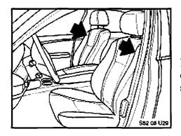
Note: This repair will be performed on the heating elements located on the outboard side of the front seats.
