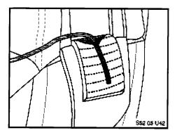
16. Twist the wires together tightly to form one slender splice of both sets of wires.
