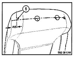
1. Fold door side backrest cover forwards and mark front foam pad (1) at the center of the head restraint holes and at a distance equal to dimension A6 from the edge.
