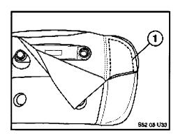
5. Draw guide lines (1) on the door side approximately 20 mm in from the seams on the padding. Then, using a seam ripper, cut along the guide lines into the fleece padding.
