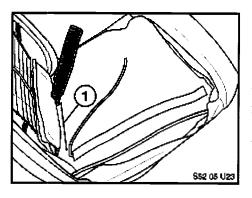
7. Cut a shallow incision (1) approximately 1/3 of the way across the bottom of the foam pad to be able to route the blue wire. Push the wire into the incision.
