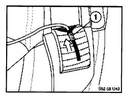
17. Push the crimp from the kit over the twisted strands with the larger diameter first.
