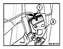
17. Crimp (1) using special tool (2) number 52 0 100. Cut off the protruding strands end of the sleeve.
