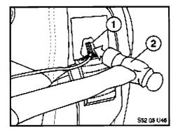
19. Using a hot glue gun, apply glue to small fleece adhesive strip (1) and affix crimped strands to the glue.
