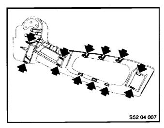
Note: For correct installation, the retaining clips must not be damaged.
