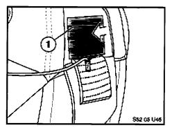
19. Affix the small fleece adhesive strip (1) (60 mm x 40 mm), from the repair kit over the padding where the cut was made.
