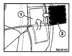
21. Fold up the first ply of the backrest heating pad (1) over the cutout. Affix another small fleece adhesive strip (2) from the kit over the cutout and the backrest heating ply.
