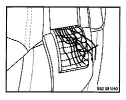
14. Once the 11 metal strands are released from the material, fan out the strands to make them ready to splice with the wire from the repair kit.
