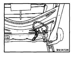
15. Insert the wiring connector's locking tab into the hole from the backside of the seat frame. Route wiring behind the backrest frame.
