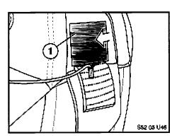
18. Affix the small fleece adhesive strip (1) (60 mm x 40 mm), from the repair kit over the padding where the cut was made.
