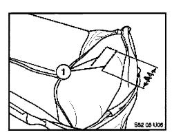
8. From the corners of the cut made for dimension A3, cut parallel incisions (1) to the left and right of the metal strands (A4) using a seam ripper.
