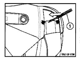
10. Using a seam ripper, carefully cut open the backrest heating pad along the marking (dimension A4) to expose all 11 metal strands. Widen the cut if necessary.
