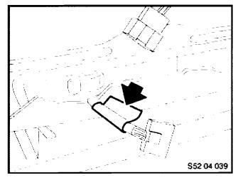
5. As indicated by the arrow, check the part number label attached to the seat heating wiring harness.
