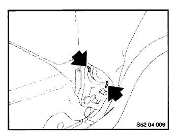
8. Unclip the door side backrest cover from the securing points at the bottom of the backrest (on the seat cushion).
