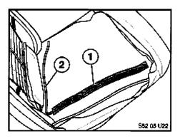
6. Affix long felt adhesive strip (500 mm x 40 mm) (1) to the outside edge in rear foam pad (above the line exit), secure blue wire to the center of long felt adhesive strip and route it downwards and towards the center of the seat (2).
