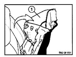
3. After removing all of the round latch clips, detach the backrest cover (1) from the foam pad. The cover will remain attached on the inboard side of the seat. Note: Passenger seat shown for the E60 (5 Series) repair.
