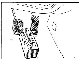
Note: A support (90 mm or 3.5 inches) under the accelerator pedal will ease cable tension and aid in disassembly
