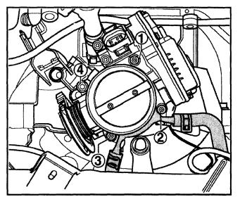
Remove throttle body from intake manifold by removing screws -1-, -2-, and -3- with a 5 mm hexagon socket; screw -4- with an 8 mm hexagon socket
