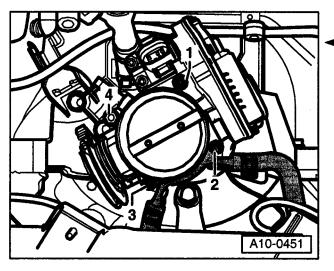
Remove throttle body from intake manifold by removing screws -1-, -2-, and -3- with a 5 mm hexagon socket and screw -4- with an 8 mm hexagon socket.
