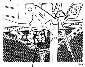
INSPECT THE PRESENCE OF WHITE SILICON AT BOLT HEAD, END OF BOLT, ON TOP OF, AND SURROUNDING SURFACES OF CRASH ZONE SENSOR
