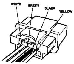
Using Terminal Tool A from the SRS Terminal Tool Set, remove the lock tab from the cable reel connector.
