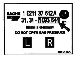
Note the part number of both front struts as shown by the arrow in the illustration. Compare the part numbers found on both front spring struts to the list below.
