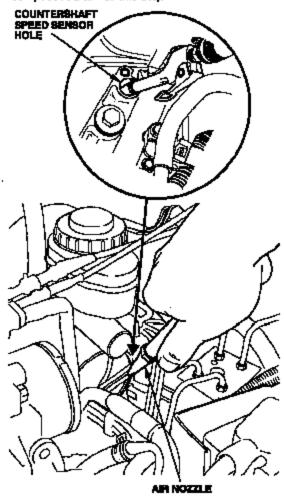
Using a clean shop tower, wipe out the bore of the countershaft epeed sensor hole.  Shine the LED flashlight into the speed sensor hole. Using a small, flat-tip screwdriver, acrape across the top of the gear teeth. This will help you get a clearer photo of the gear.
