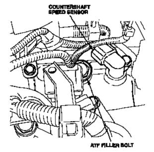
Remove the countershaft speed sensor. Refer to page 14-128 of the service manual.  Connect an air nozzle to the shop air supply. Insert the air nozzle into the countersheft speed sensor hole, and apply air to the top of the second gear for for at least 15 seconds.
