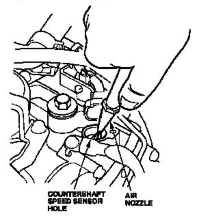
Using a clean shop towel, wipe cut the bore of the countershaft speed sensor hole.  Shine the LED flashfight into the speed sensor hole. Using a small, flat-tip ecrewdriver, scrape across the top of the geer teeth. This will help you get a clearer photo of the gear.
