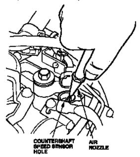
Using a clean shop towel, wipe out the bore of the countershaft speed sensor hole.  Shine the LED flashlight into the speed sensor hole. Using a small, flat-tip screwdriver, scrape across the top of the gear teeth. This will help you get a clearer photo of the gear.
