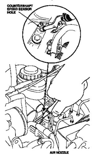
Using a clean shop towel, wipe out the bore of the countershaft speed sensor hole. Shine the LED flashlight into the speed sensor hole. Using a small, flat-tip corewortver, sorape across the top of the gear teeth. This will help you get a clearer photo of the gear.
