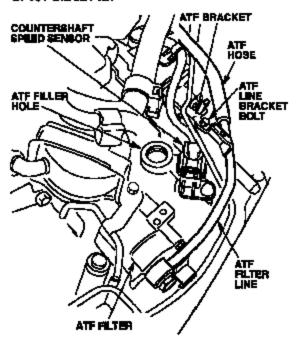
Remove the filter line bracket bott, then remove and discard the ATF filter line assembly.
