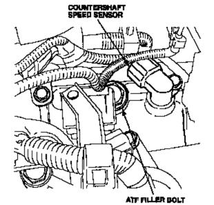
Remove the countershaft speed sensor, For Odyssey, refer to the 1999–04 Odyssey Service Manual, page 14-134. For Pilot, refer to the 2003–04 Pilot Service Manual, page 14-123.  Connect an air nozzle to the shop air supply. Insert the air nozzle into the countershaft speed sensor hole, and apply air to the top of the second gear for at least 15 seconds.
