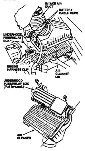
Remove the two 10 mm bolts from the under-hood fuse/relay box. Then detach the engine harness clip from the fuse/relay box, and pull the fuse/relay box forward. Clean the area around the ATF filler bolt, the countershaft speed sensor, and the ATF filter lines.
