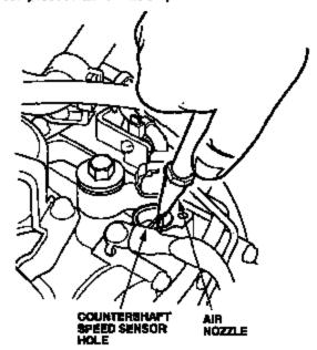
Using a clean shop towel, wipe out the bore of the countershaft speed sensor hole.  Shine the LEO flashlight into the speed sensor hole. Using a small, flat-tip screwdriver, scrape across the top of the gear teeth. This will help you get a clearer photo of the gear.
