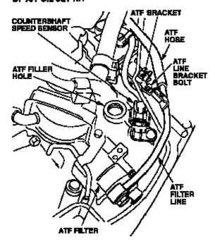
Remove the filter line bracket bolt, then remove and discard the ATF filter line assembly.
