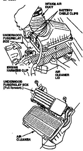
Remove the two 10 mm bolts from the under-hood fuse/relay box. Then detach the engine harness clip from the fuse/relay box, and pull the fuse/relay box forward. Clean the area around the ATF filler bolt, the countershaft speed sensor, and the ATF filter lines.
