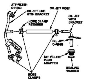
Install the cil jet line on the ATF hose with a new hose clamp.
