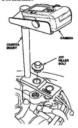
12. Attach the camera to the camera mount. Make sure the camera spacer is correctly installed, and be careful not to damage the plastic threads in the bottom of the camera. 13. 9.2CL and 3.2TL: Detach the throttle cable from the cable stay on the driver's side of the bulkheed. Bafore taking any photos, move the throttle cable and the purge control hose out of the way. 2004 TL: Make sure the fuse/relay box is out of the way.
