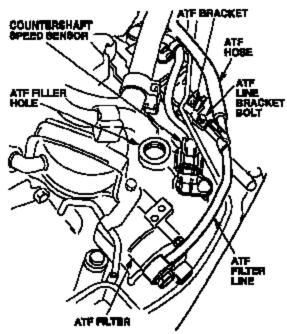
Remove the fitter line bracket bolt(s), then remove and discard the ATF fitter line assembly.
