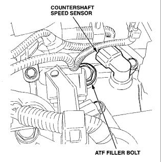
Remove the countershaft speed sensor. For Odyssey, refer to the 1999–04 Odyssey Service Manual, page 14-134. For Pilot, refer to the 2003–04 Pilot Service Manual, page 14-123. On ISIS, use the keywords "count sen." and select A/T Output Shaft (Countershaft) Speed Sensor Replacement from the list.  Connect an air nozzle to the shop air supply. Insert the air nozzle into the countershaft speed sensor hole, and apply air to the top of the second gear for at least 15 seconds.
