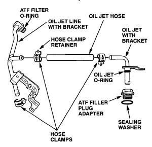
8. Install the oil jet line on the ATF hose with a new hose clamp.
