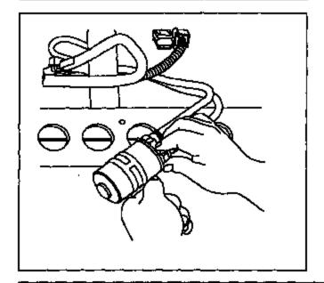
Tilt the fuel filter downward and drain off the fuel into an approved fuel container. Disconnect the fuel tank feed and return hose fittings from the fuel filter. Refer to Steps 7.1 – 7.5 for instructions for disconnecting quick connect fittings (plastic collar – press release).
