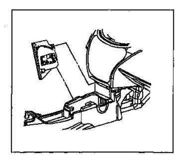
6.3 Install the console side extension retainer and turn clockwise to secure.
