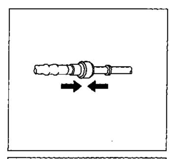
3.2 Push both sides of the fitting together to cause the retaining tabs to snap into place.
