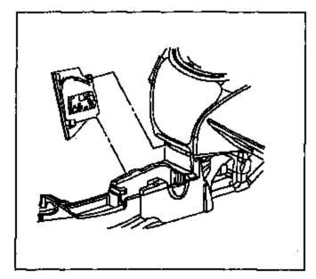
2.2.3 Locate fuel pump relay in BCM fuse box. Remove fuel pump relay. Place fuel pump relay in a safe location. Do NOT discard fuel pump relay.
