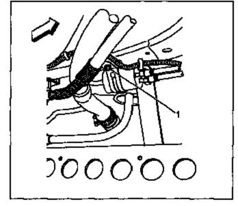
Disconnect the fuel filter from the engine fuel feed pipe (1). Refer to Steps 5.1 – 5.5 for instructions for disconnecting quick connect fittings (metal collar).
