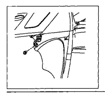
2.2.2 Remove the left console side extension by pulling the console side extension rearward to disengage from the console.
