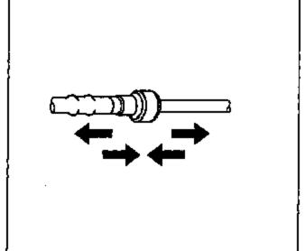
3.3 Once installed, pull on both sides of the fitting to make sure the connection is secure.
