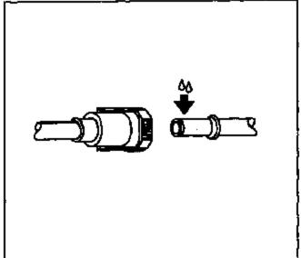
CAUTION: In order to reduce the risk of fire and personal injury, before connecting fuel pipe fittings, always apply a few drops of clean engine oil to the male pipe ends. This will ensure proper reconnection and prevent a possible fuel leak. During normal operation, the O-rings located in the female connector will swell and may prevent proper reconnection if not lubricated.
