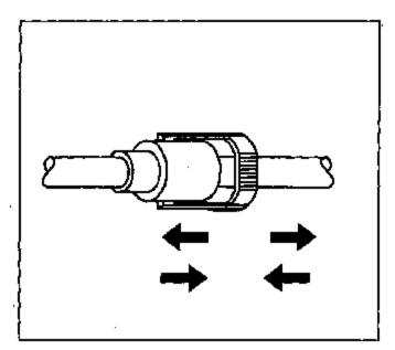
Connect the fuel filter to the engine feed fuel pipe (1). Refer to Steps 3.1 - 3.3 for instructions for connecting quick connect fittings (metal collar).
