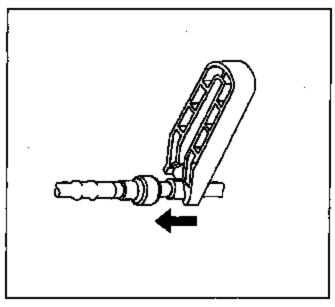
5.2 Choose the correct tool from J 37088-A tool set for the size of the fitting. Insert the tool into the female connector, then push inward to release the locking tabs.
