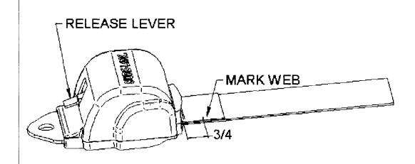
6 clicks to retract 3/4" of fully-extended web identifies a properly functioning retractor 12 clicks to retract 3/4" of fully-extended web identifies a defective unit that requires replacement
