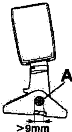
Figure 2 The axle pin of the single and double belt buckle is riveted correctly, if the measured rivet head diameter (Figure 2, Item A) is 9 mm or larger.
