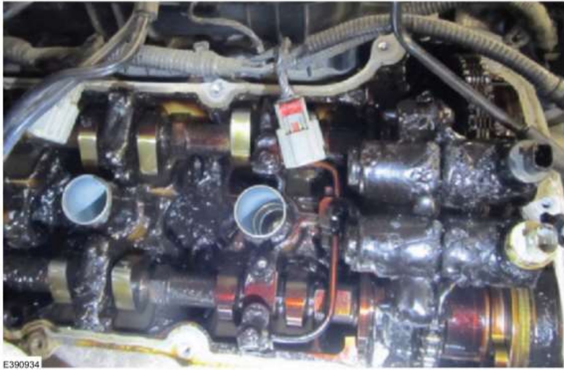
Heavy oil sludge build-up on the underside of the valve cover. (Figure 9)
