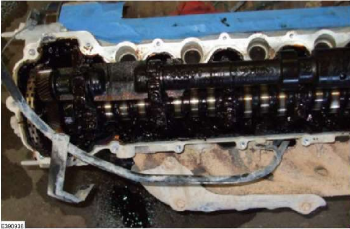
Heavy oil sludge on the underside of the valve cover. (Figure 13)
