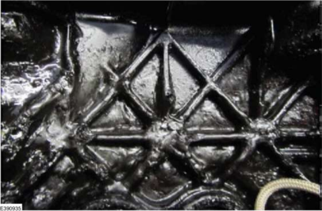
Sludge accumulation on the valvetrain and oil pick up tube. Oil is thick and broken down, show significant signs of lubrication restriction from sludge accumulation. (Figure 10)
