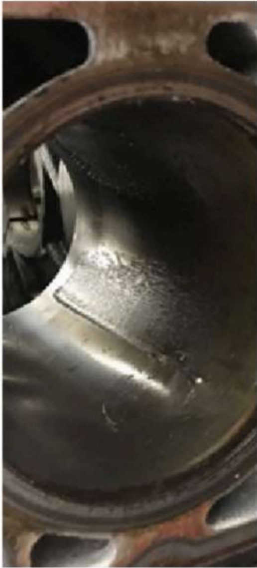
Piston Skirt – Normal Wear: Light wear of the coating (Figures 44-45). Figure 44
