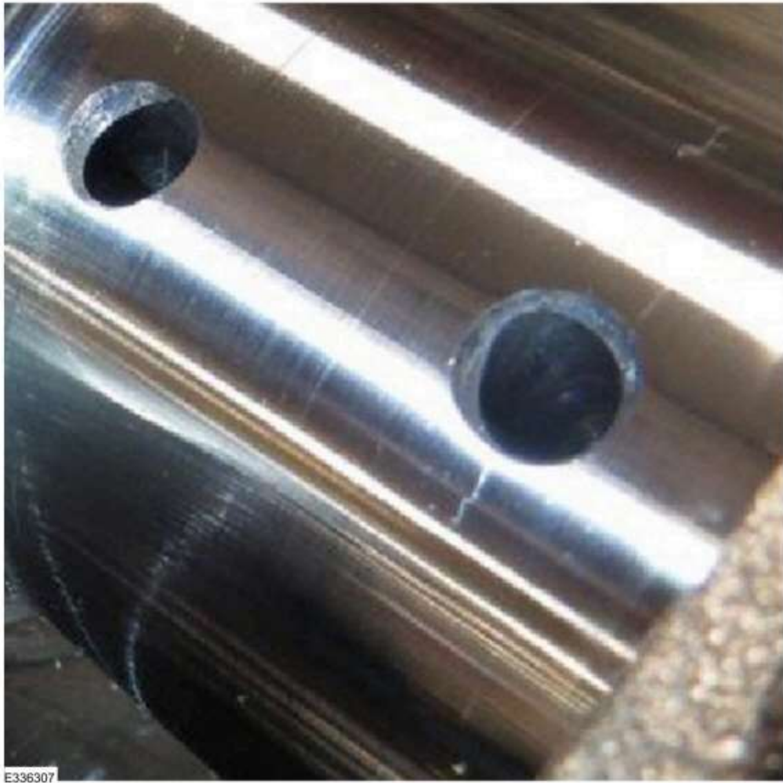
Crankshaft – Damage: Material loss, deep scoring, material transfer (Figures 30-32).
