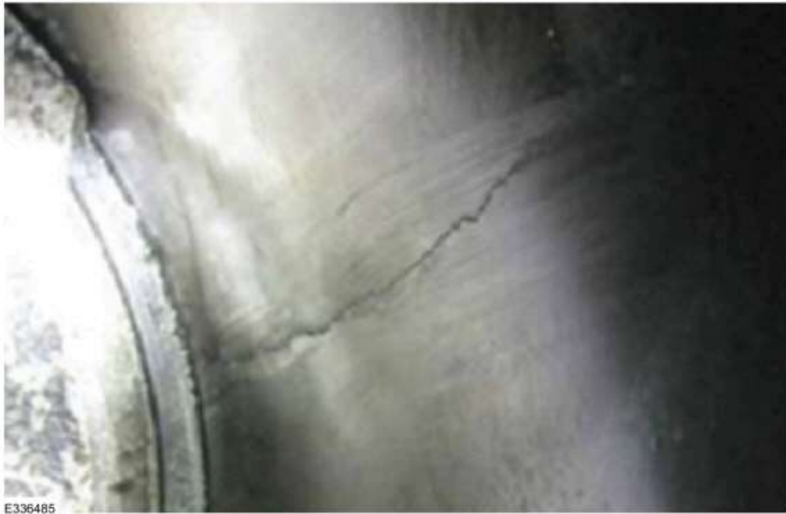
Excess detonation causes excess cylinder pressure spikes leading to piston ring land fractures (second ring land is damaged). (Figure 52)
