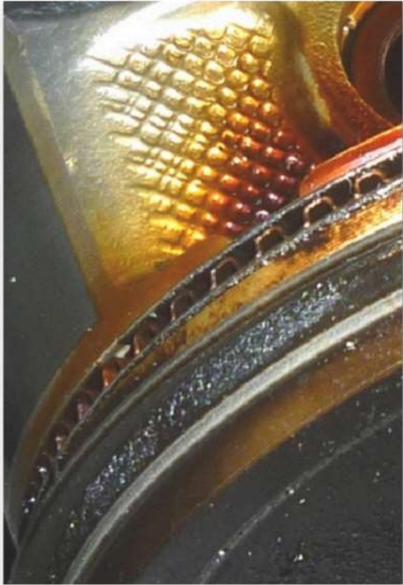
Valve Damage (Figures 56-57)
