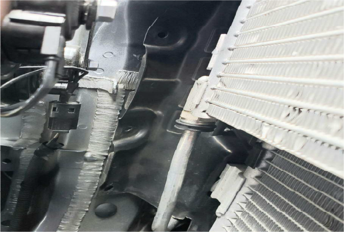
22B. Same rubber flange from above showing missing fasteners.
