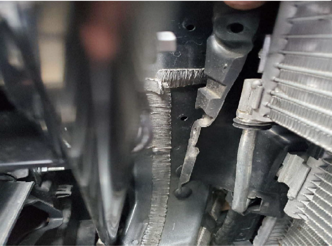
22B. Same rubber flange from above showing missing fasteners.
