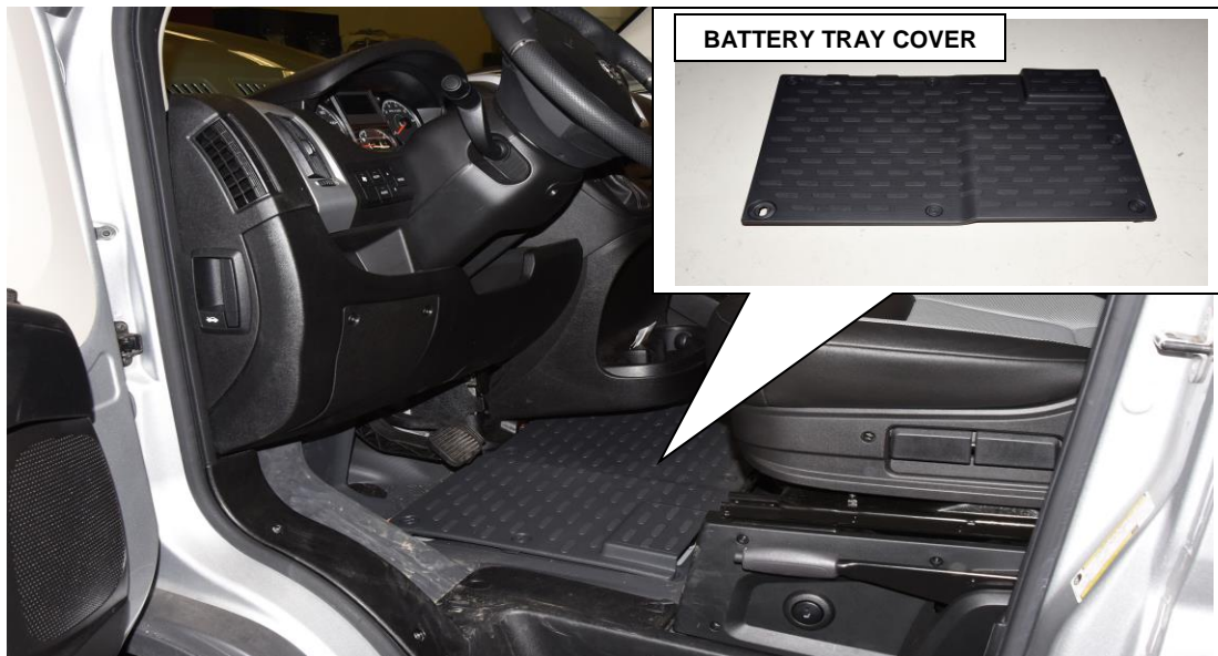
Figure 24 – Battery Tray Access Cover
