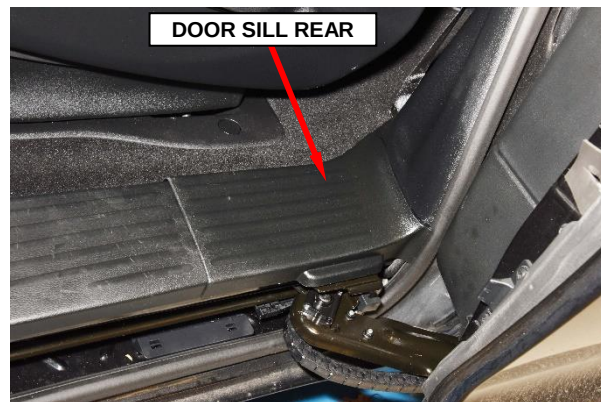
Figure 22 – Door Sill Rear
