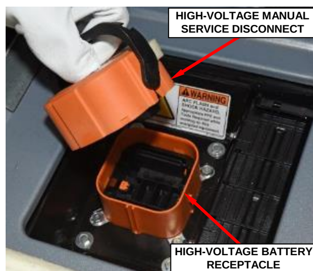
Figure 12 – High-Voltage Manual Service Disconnect and Receptacle
