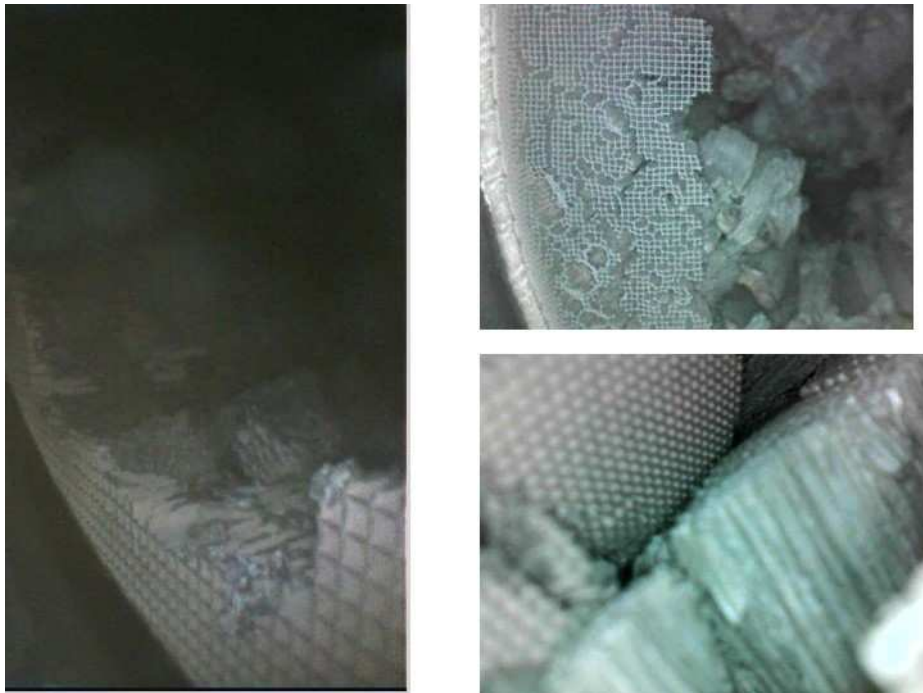
Fig. 5 Extreme Damaged Substrate
