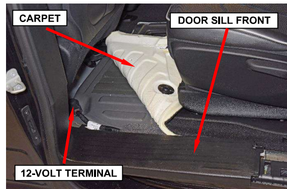
Figure 22 – Door Sill Front and Carpet
