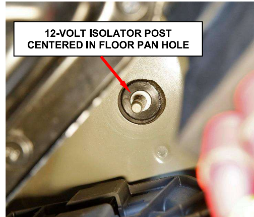
Figure 28 – 12-volt Isolator Post with Attached Guide Removed
