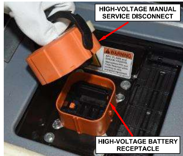
Figure 12 – High-Voltage Manual Service Disconnect and Receptacle
