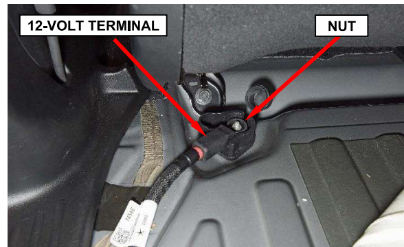
Figure 24 – 12-Volt Cable Terminal
