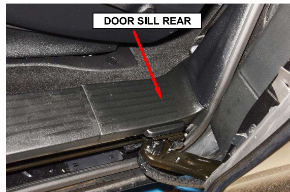
Figure 21 – Door Sill Rear
