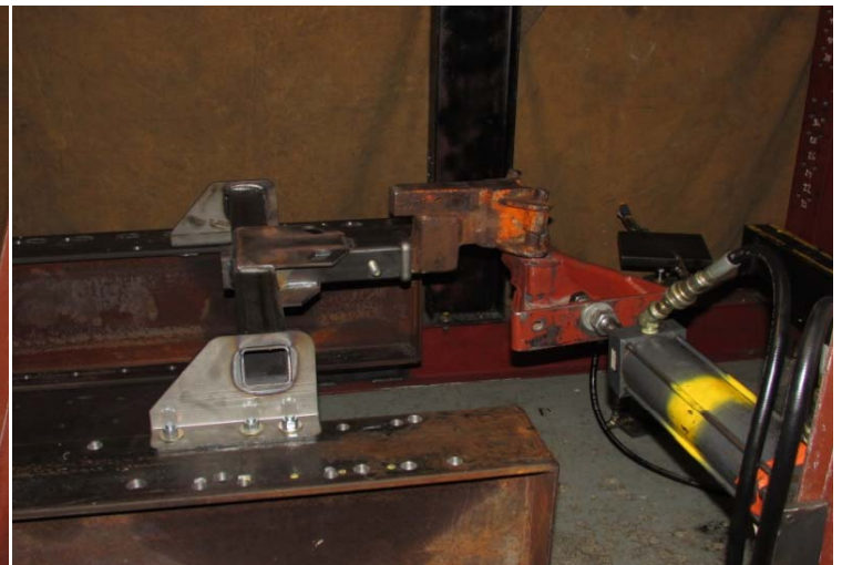
Step E - Full Load Applied
