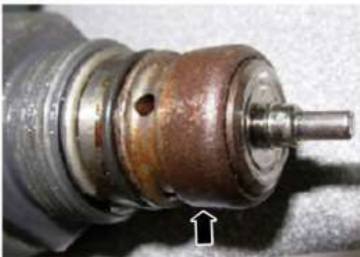
Figure 17 - Rust staining on VCV screen
