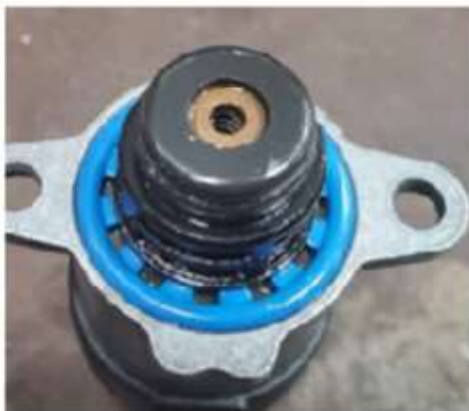
Figure 19 - Contamination on the end of the VCV
