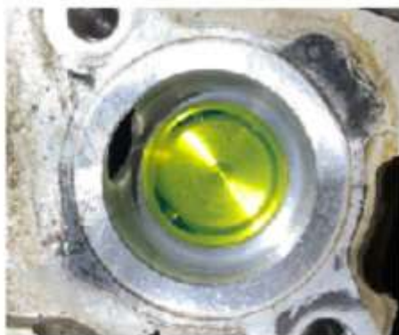
Figure 6 - Small particle in the VCV port
