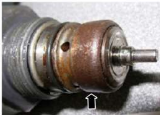
Figure 17 - Rust staining on VCV screen
