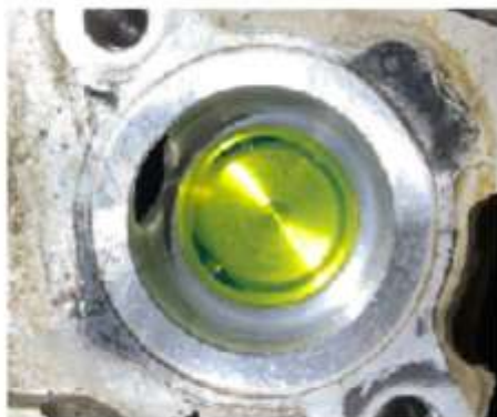
Figure 6 - Small particle in the VCV port
