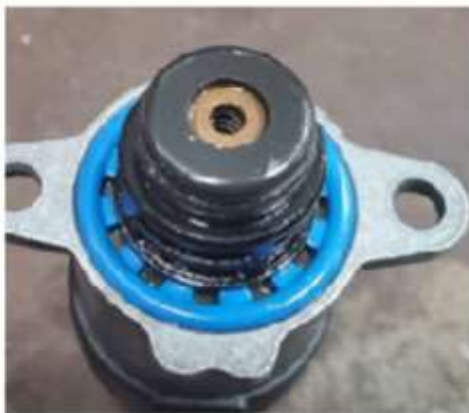
Figure 19 - Contamination on the end of the VCV
