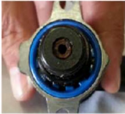
Figure 16 - Rust on the fuel side of the PCV
