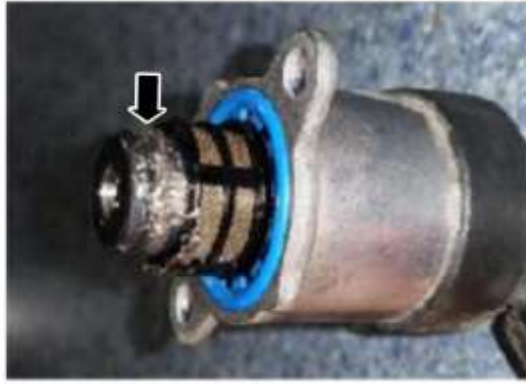
Figure 18 - Bio growth on the end of the VCV
