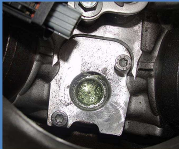
VCV port in the HP Fuel Pump
