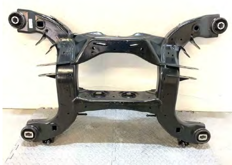
Fig. 1 – Rear Subframe Assembly with Two Rear Axle Mounting Bolts
