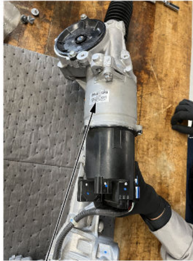
BARCODE Install with barcode facing up.
