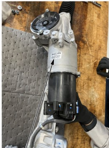
BARCODE Install with barcode facing up.
