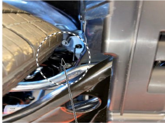
INNER TIRE CONTACT WITH LOWER ARM AND/OR OUTER TIE ROD
