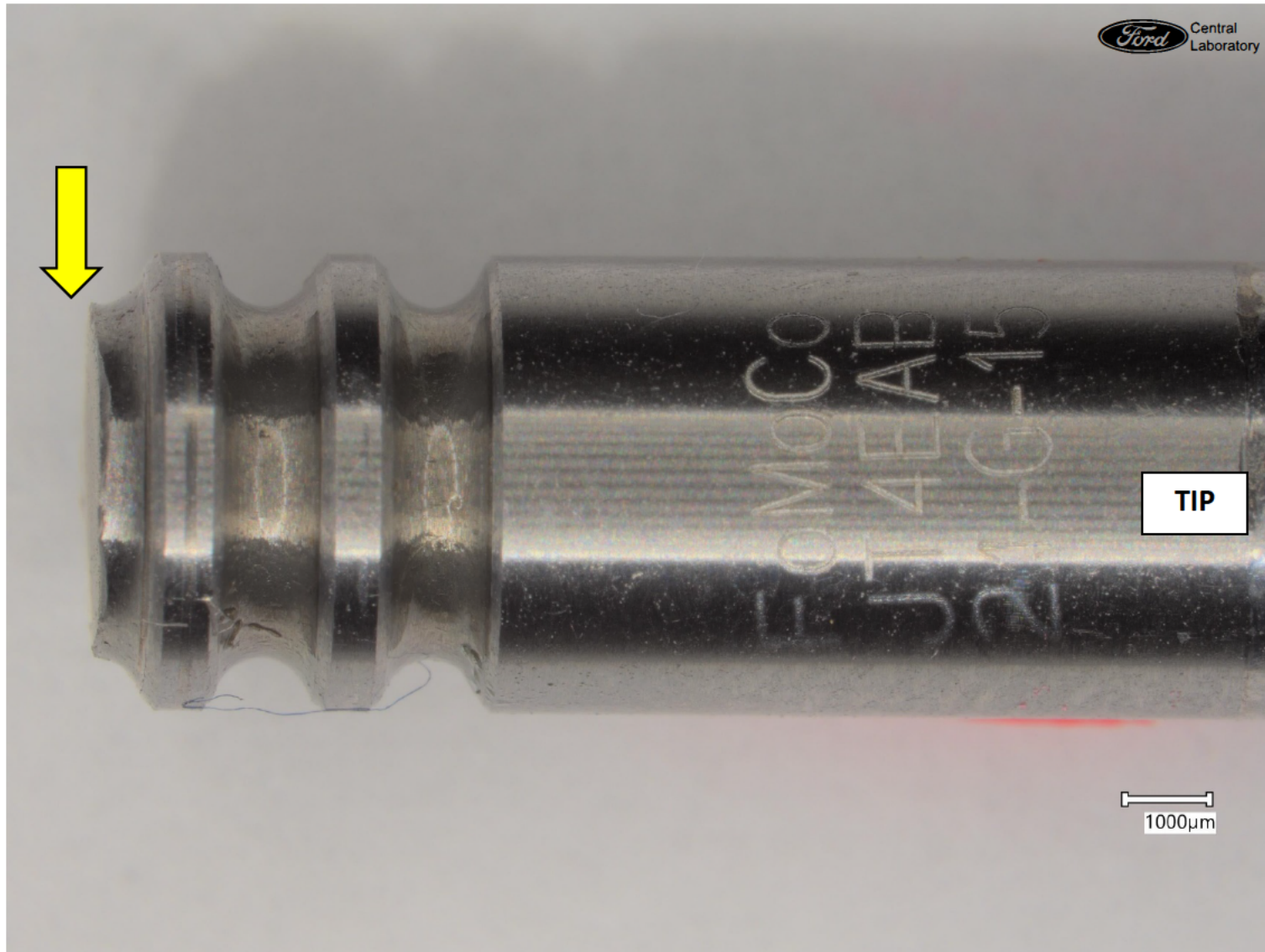
Figure 4: Intake Valve – 12 – Magnified view of Figure 2 showing the fracture at the third keeper groove from the tip, indicated by the yellow arrow.
