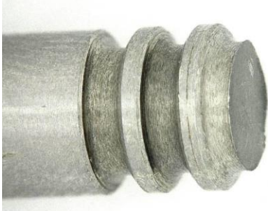
Figure 1: Tip Fracture in 3 rd Keeper Groove
