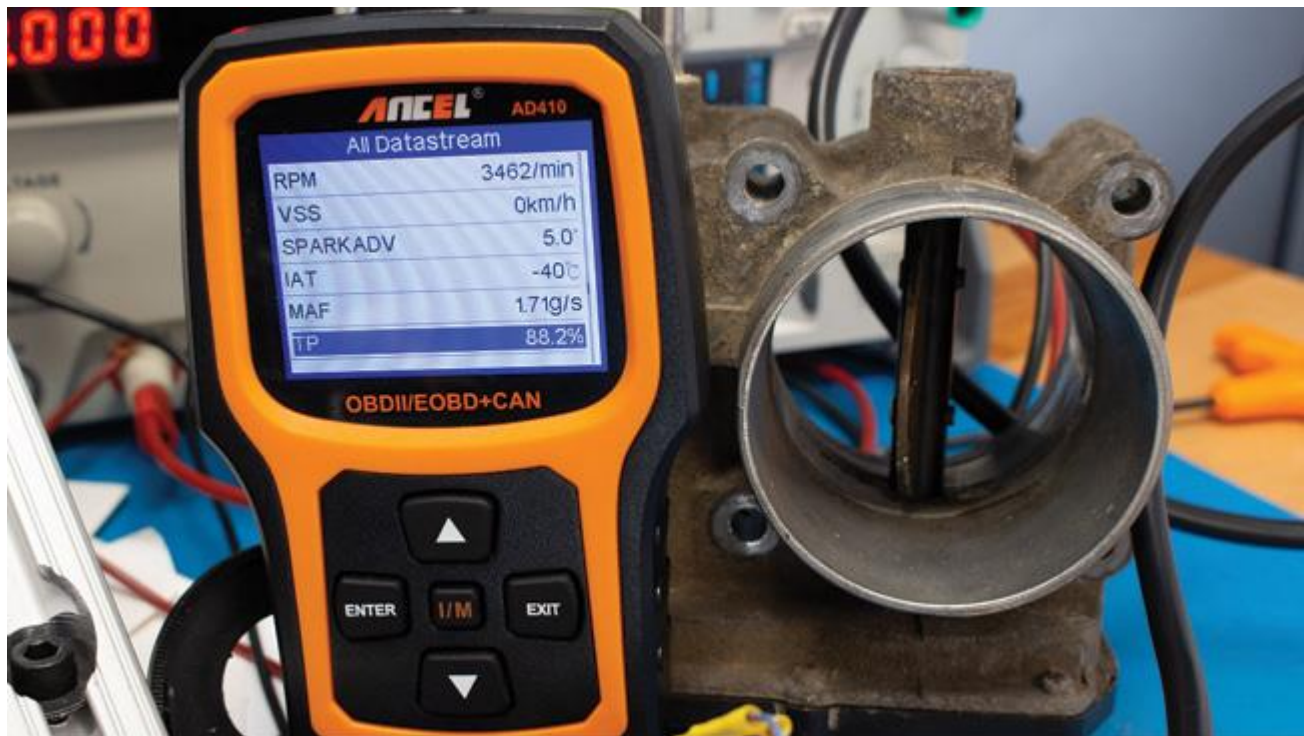
Figure 52 – Wide Open Throttle and ODB-II reader showing that the throttle is commanded to 88%. The motor is being actively driven with a constant “on” voltage (no PWM operation is observed). [This constant “on” voltage may be just a 100% PWM duty cycle].
