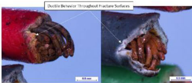
Figure 5. Fractured wire ends from warranty harnesses.
