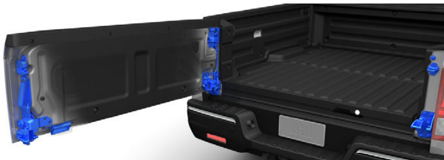
Horizontal (“swinging”) tailgate action
