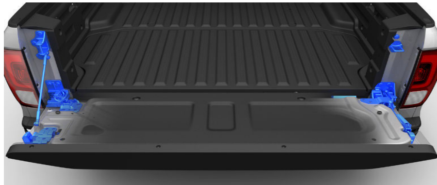
Vertical (traditional pick-up truck) tailgate action
