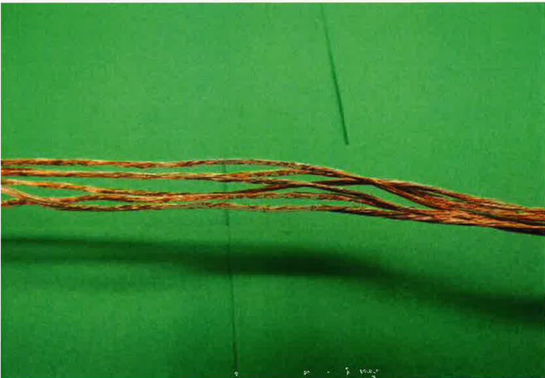
Figure 24 - Wire Harness Assembly #1 - General Mode Post Durability Cycling - Flex Area - Insulation Removed - No Breakage
