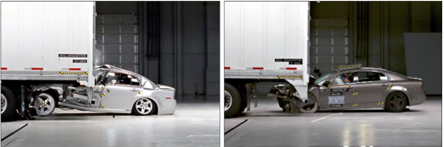
Figure 1: Crash Tests of Rear Guards with (left) and without (right) Passenger Compartment Intrusion
