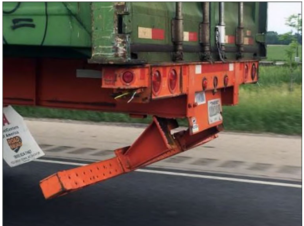
Figure 5: Example of a Damaged Rear Guard
