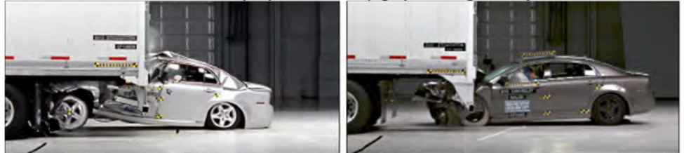
Crash Tests of Rear Guards with (left) and without (right) Passenger Compartment Intrusion
