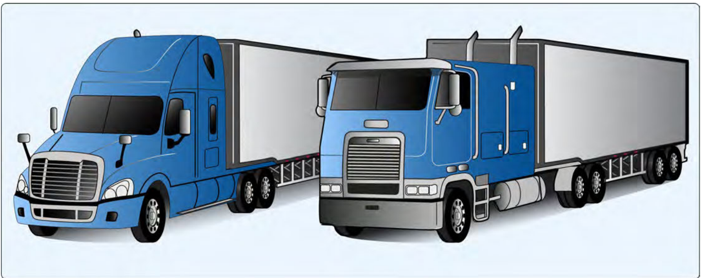
Figure 6: Examples of a Conventional Tractor (left) and Cab-Over Tractor (right)
