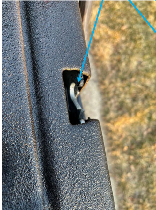
Overspray of bedliner treatment directly on latch components
