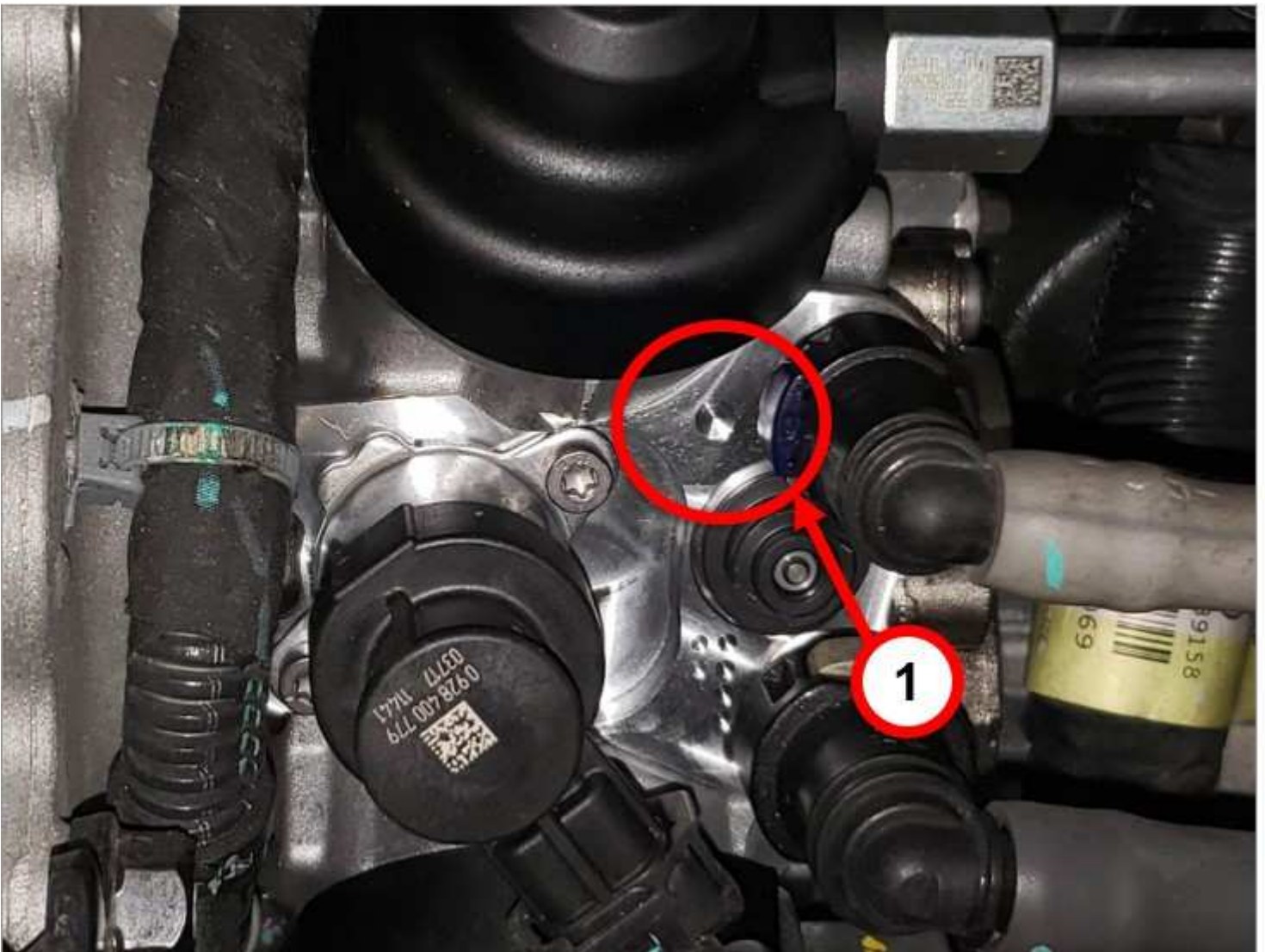
Fig. 1 New Style Symmetrical Cam Design Pump
