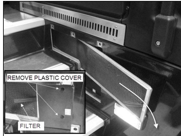
REMOVING DRIVER'S SECTION AIR FILTER
