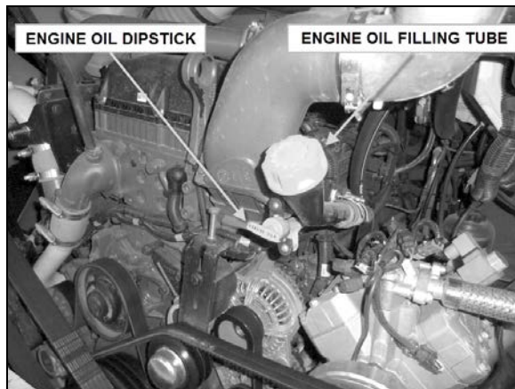
ENGINE OIL DIPSTICK - VOLVO D13 ENGINE 01192_1
