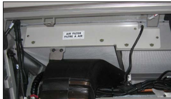
PASSENGERS AREA AIR FILTER REMOVAL
