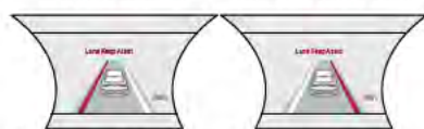
When the front camera detects the vehicle moving outside of the lane, a vehicle crossing lane indicator will flash, either on the left or right lane (as shown in both images above).
