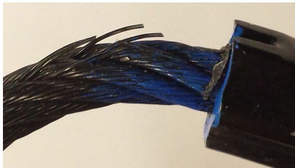
Example of cycled part from testing with visibly broken strands.
