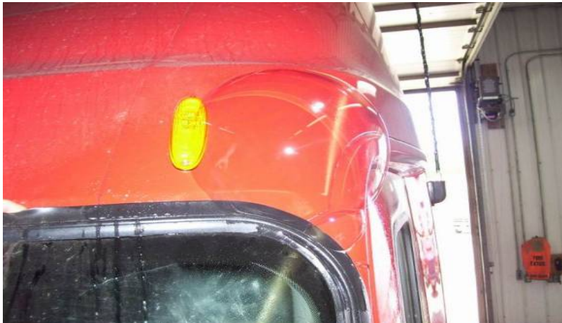
Likely leak between seal and cab OR between roof-cap and cab
