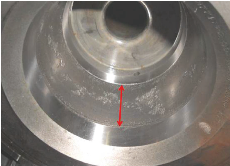
Spalled bearing race (Image 4)
