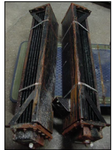
Copper Brass Radiator samples leak checked during SWAAT Test
