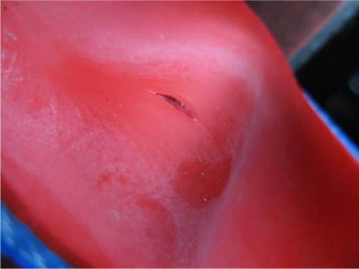
LINER BREACH POINT WITH CONTAMINATION
