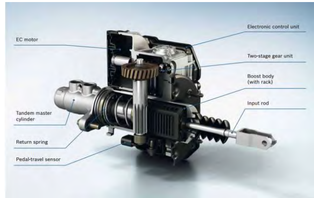
Figure 19. Cross section of the 1st gen iBooster showing the electric motor and gear drive. 16
