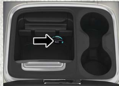
Power Outlet — Center Console
