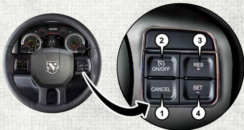
Speed Control Switches
