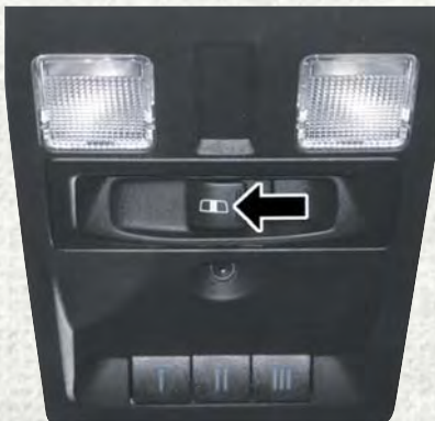
Power Sliding Rear Window Switch
