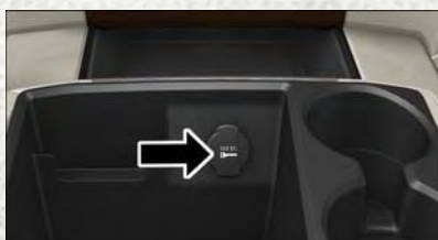
Power Outlet — Center Console
