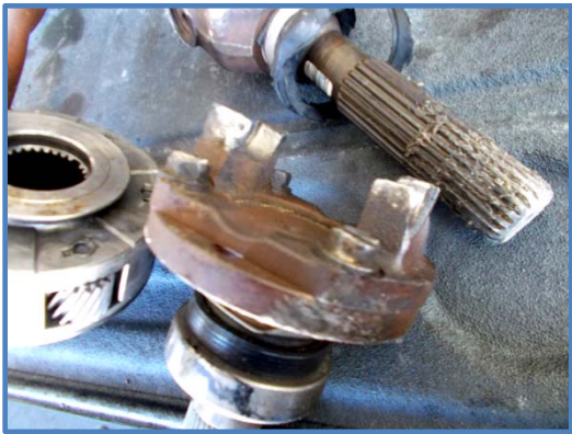
Figure 1: Expensive, broken universal joint
