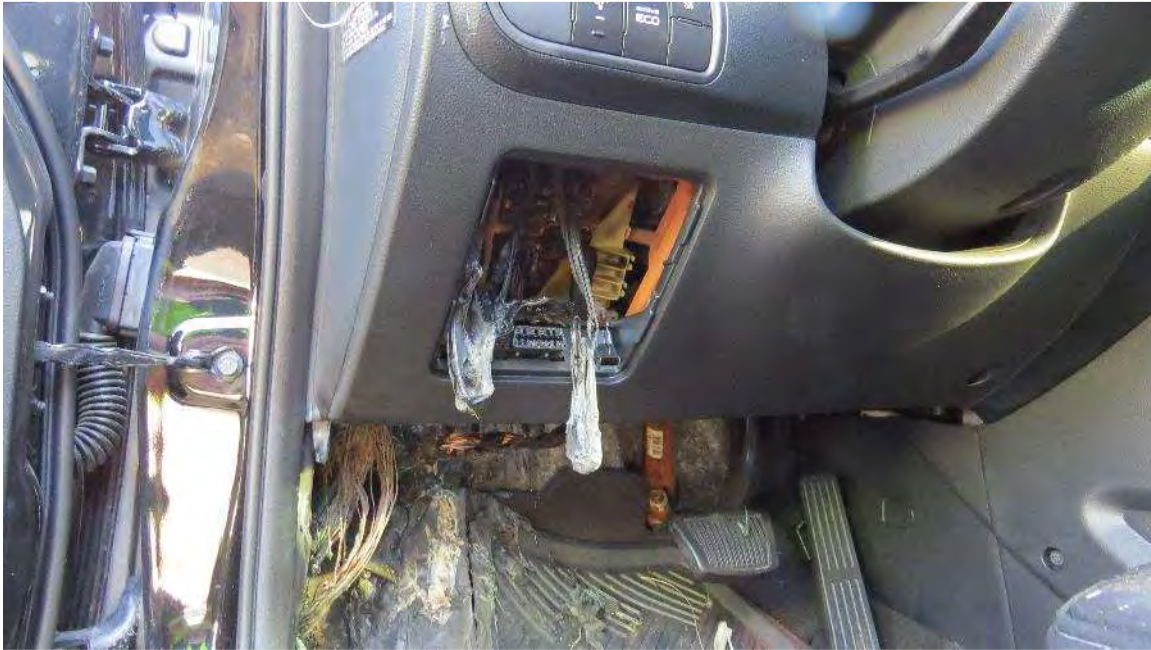
Photograph 5: Melted plastic cover for the interior fuse block. No fire damage to the OBDII connector.
