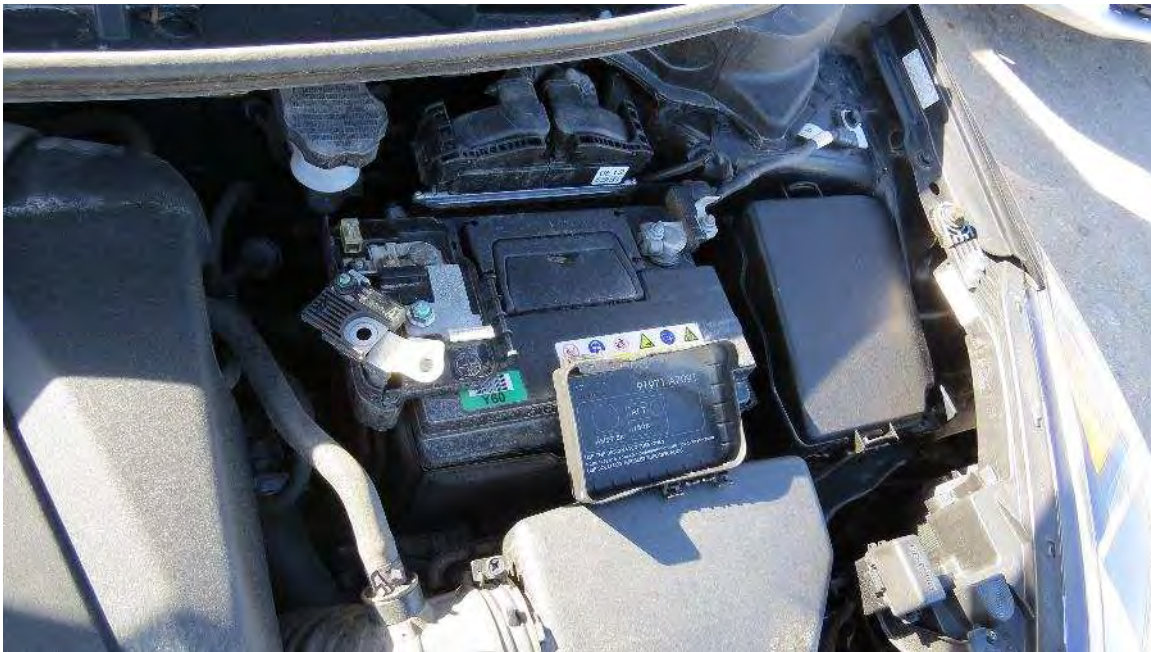
Photograph 6: Battery positive cable disconnected by the storage yard.
