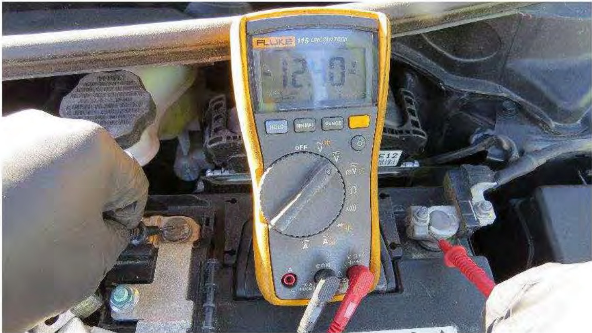
Photograph 8: Measurement of the battery voltage.
