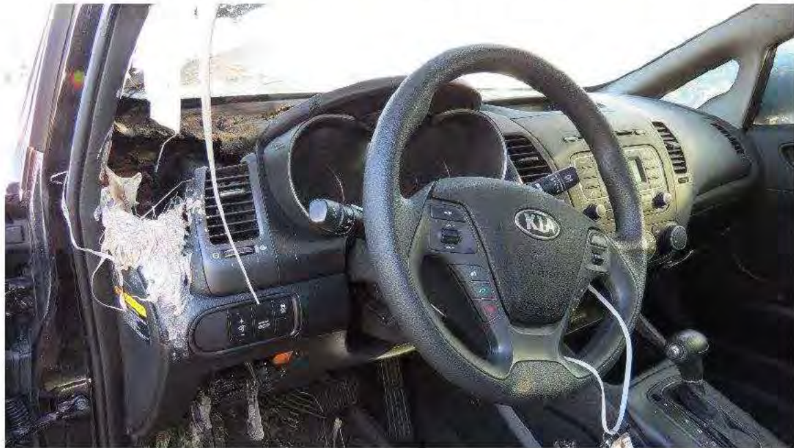
Photograph 4: Fire-damaged driver's side of the dashboard.
