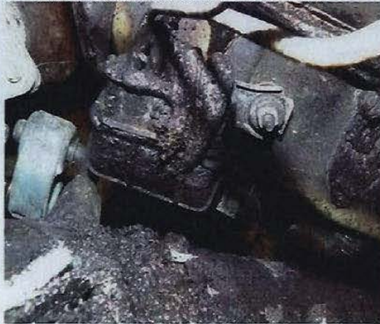
70. View of the combustible fuel line with the brake line at the bulkhead.
