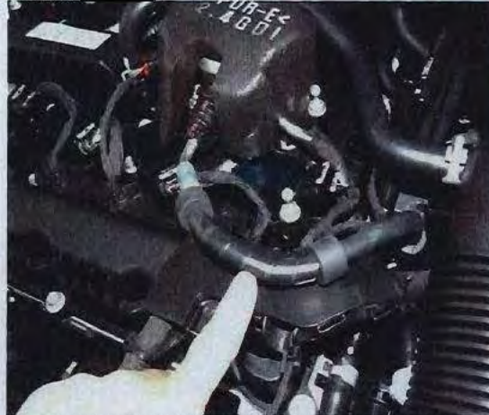
97. Another view of the supply fuel line traveling to the high pressure fuel pump.
