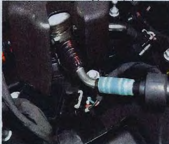
98. View of the fuel line connection to the high pressure fuel pump.
