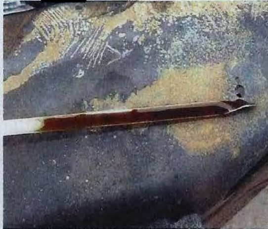
71. View of the engine oil registering over full.
