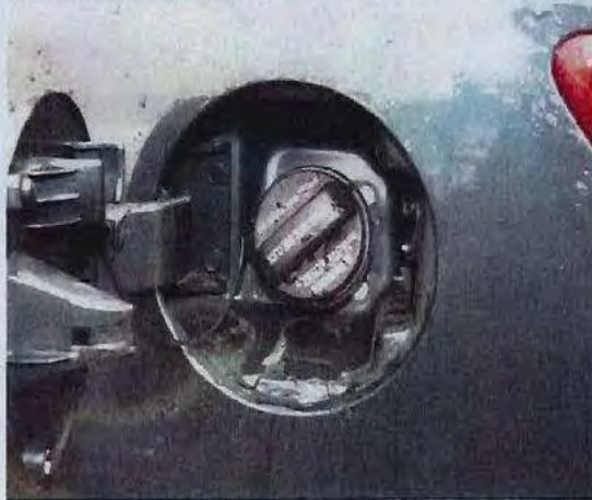
72. View of the fuel cap intact.
