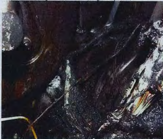
50. View of the wiring harness, left rear of the engine compartment.
