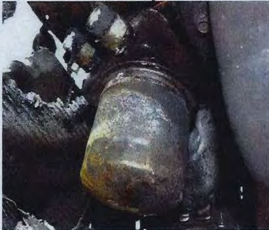
78. View of the oil filter seen from undercarriage.
