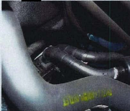
93. Another view of the routing of the fuel line at the bulkhead.
