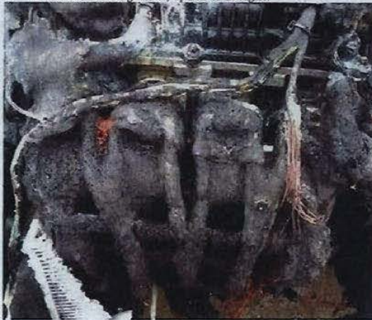
40. View of the same wiring harness, top front of the engine.
