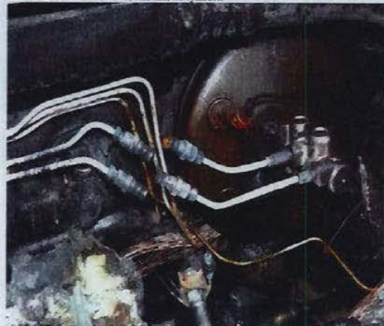
48. View of the brake lines and master cylinder.
