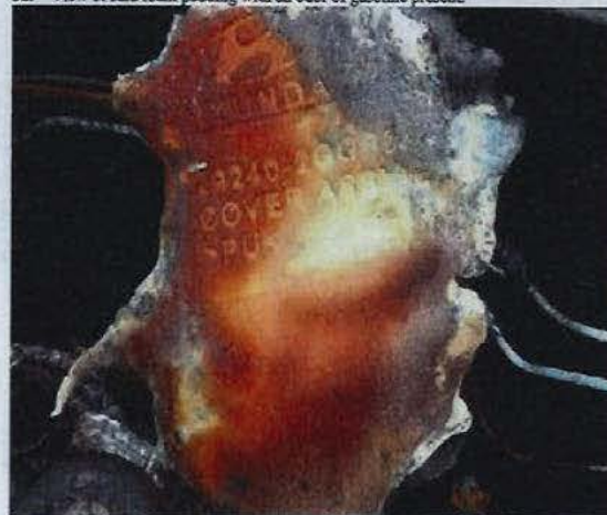
52. View of said foam padding with an odor of gasoline present.
