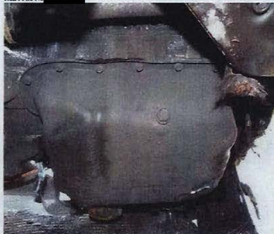
79. View of the oil pan and drain plug.
