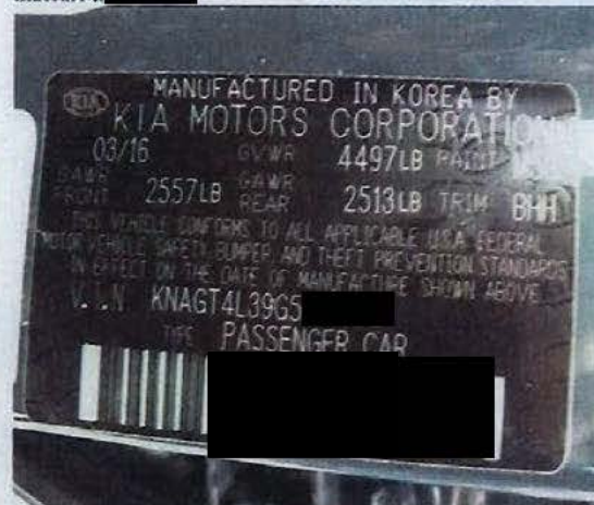
1. View of the Federal Manufacturers Label secured to the driver B-pillar.
