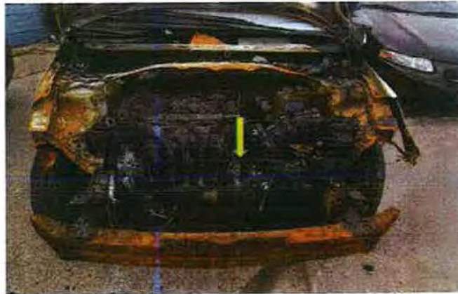
View showing the area of origin along the left side of the engine.
